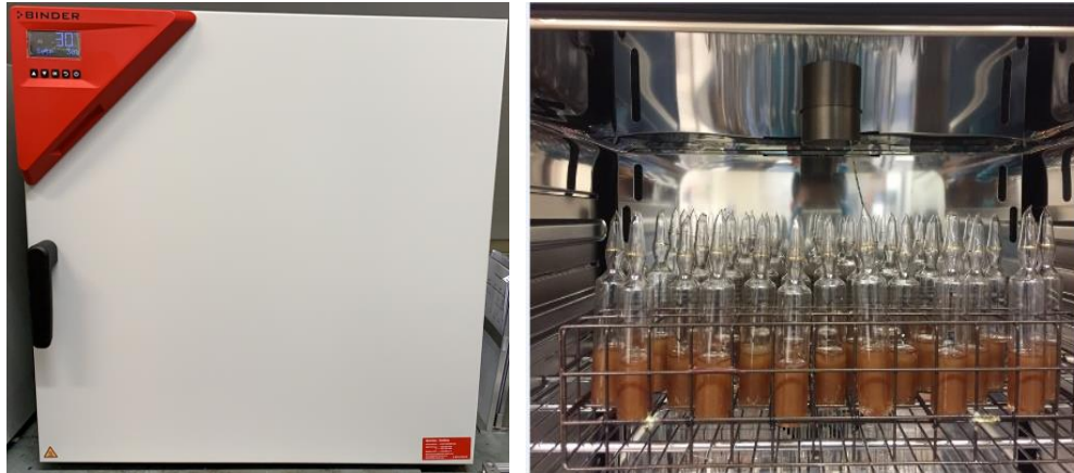
Figure 3.4 External and internal appearance of the Binder oven used for thermal ageing of the transformer insulation oil and paper.
