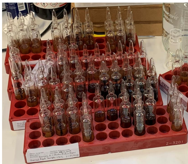
Figure 5.1 A photo of the oil-paper samples in sealed ampoules aged for different durations. It is placed in this chapter as a record of the original test samples that may contain information that is needed in future.
