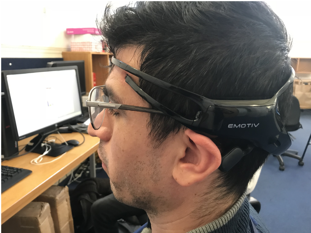
Figure 2.1. A consumer grade EEG unit: Emotiv Epoch.
