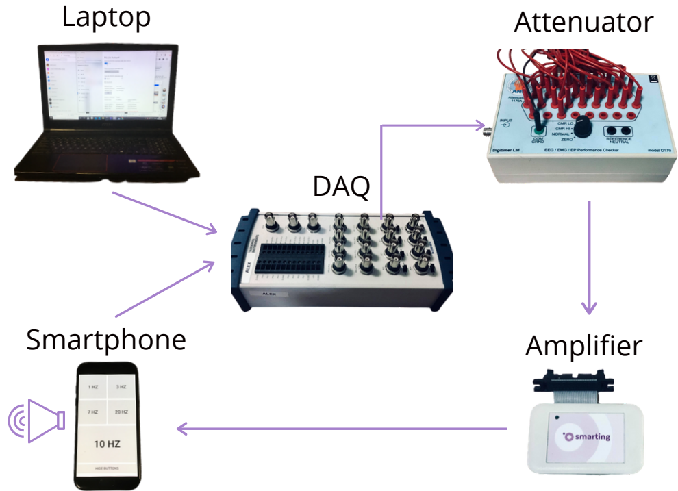
Figure 5.11. Test setup for the audio mode. EEG data streamed from the laptop is converted to an analog voltage, which is then attenuated via the attenuator before passing onto the amplifier. Note that the audio output from the phone is collected at the DAQ's input channel for recording, and is not passed onto the attenuator.
