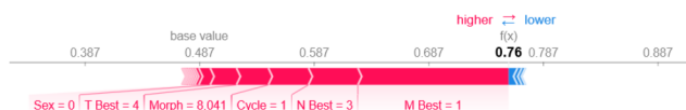
Figure 2. SHAP local explanation. The width of each descriptive block and colour are indicative of the shift in probability for the instance.
