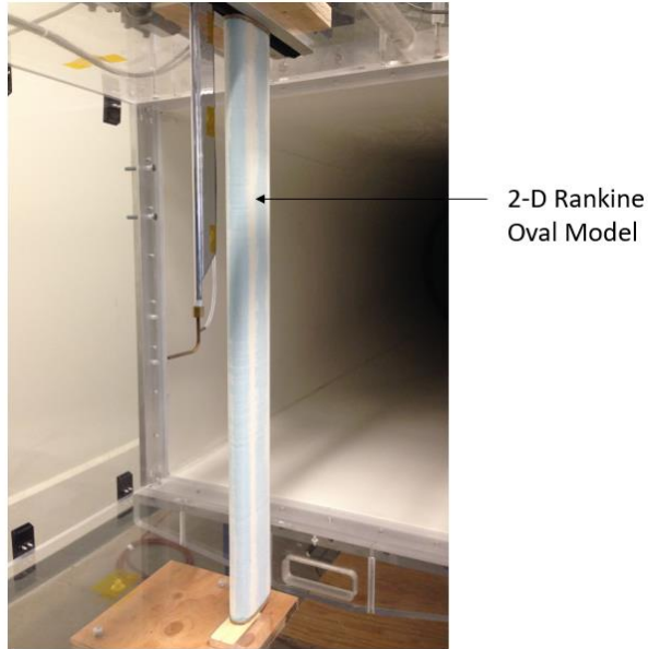
Figure 3-2: Rankine Oval Pressure Disturbance Experiment. Private Communication, 2014 30 .
