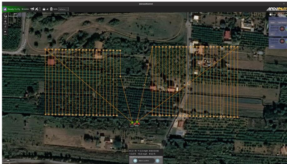
Figure 5.10: Mission planning for multiple drones with QGroundControl
