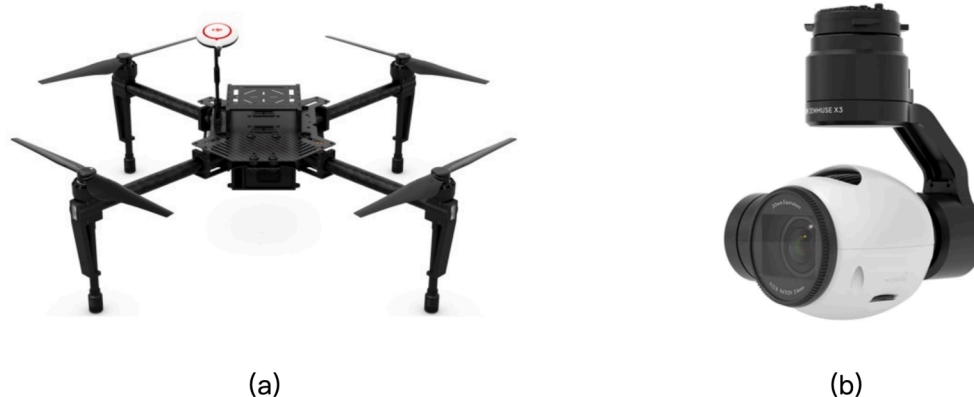
Fig. 4. The images were collected with (a) a DJI Matrice 100 UAV with (b) a Zenmuse X3 NDVI camera.
