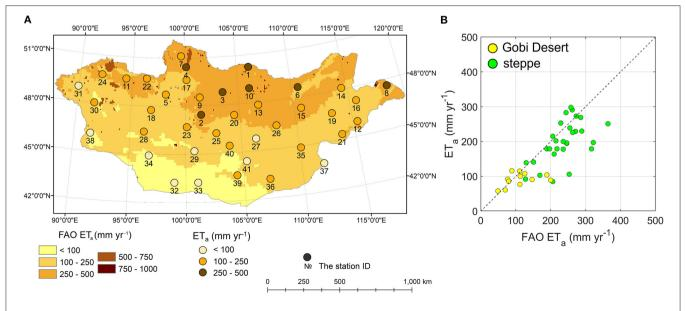
**FIGURE 3** [ET characteristics: (A) mean actual annual evapotranspiration (ET<sub>a</sub>) simulated in HYDRUS-1D (black dots) over the 41 weather stations on the FAO map; and (B) comparison between ET<sub>a</sub> values reported in the FAO map (FAO ET<sub>a</sub>) and ET<sub>a</sub> values simulated in HYDRUS-1D (ET<sub>a</sub>). Green and yellow circles indicate the steppe region and Gobi Desert, respectively.
