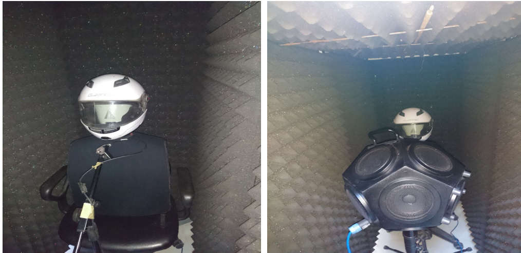
Figure 1 - Experimental setup; the cabinet, the head-torso simulator, the 4189-A-021 type microphone and the omnidirectional sound source.
