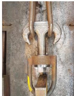
Figure 2-14. Crane hooks manufactured using WAAM by Huisman (Kanaris, 2018)
