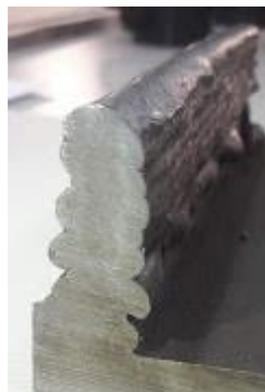
Figure 3-14. Variation in the thickness and surface roughness up the printed wall.
