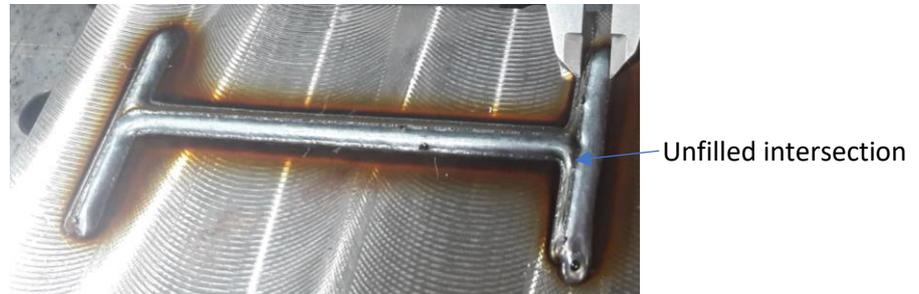
Figure 3-27. A printing path without the mid bead for the web and the unfilled interaction.
