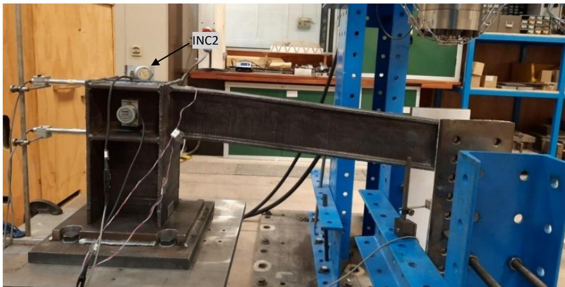
Figure 6-19. Printed beam-to-column joint after its deflection reached 80mm
