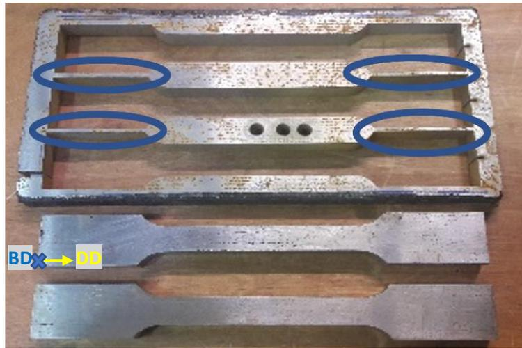
Figure 4-7. Autodesk plate: Location of the straight sided (circled blue) specimens extracted from the leftover material
