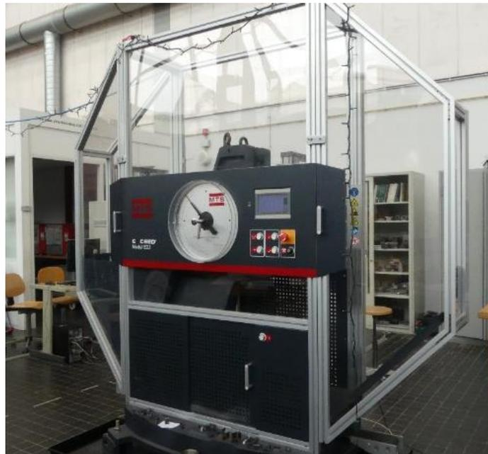
Figure 4-30. MTS Exceed E22 pendulum impact testing machine in the TU-Delft lab
