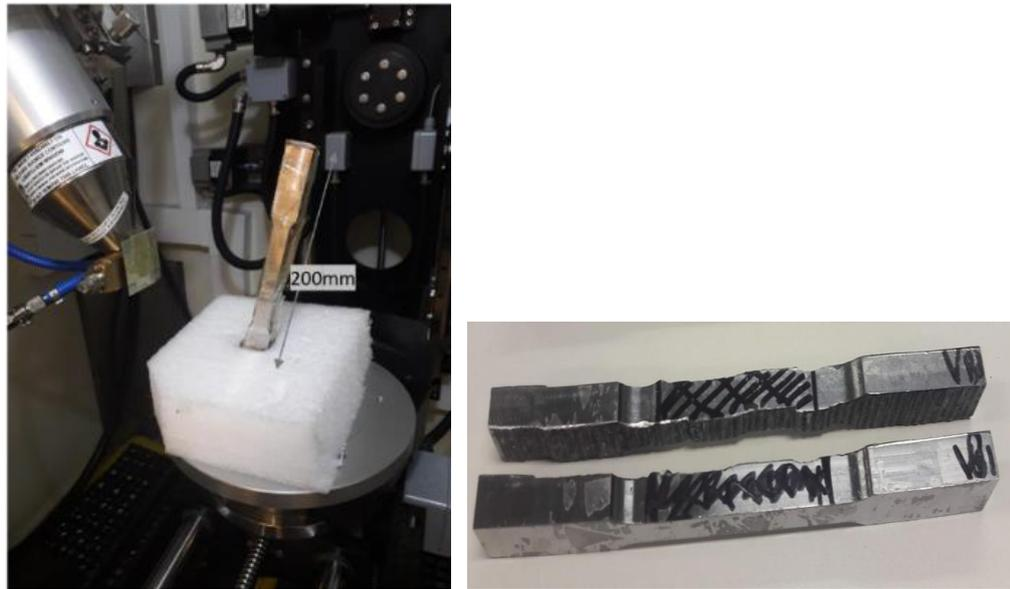
Figure 4-44. (a) Dog-bone coupon; (b) volume of interest marked on surface with black pen marks
