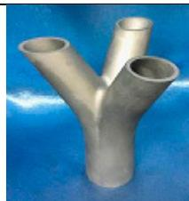
Figure 2-19. Trifurcated stainless-steel joint (He et al., 2020)
