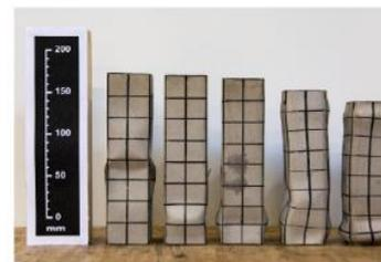
Figure 2-16. Stainless-steel printed SHS stub columns (Buchanan et al., 2017)
