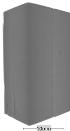
Figure 4-45. X-CT image of an EN 8 steel specimen used as a benchmark.
