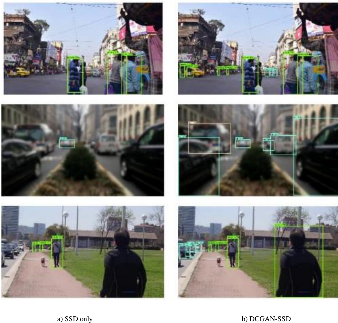
Figure 4.2 Detection results for the comparison between a) detection performed only with SSD, b) detection performed by DCGAN-SSD.
