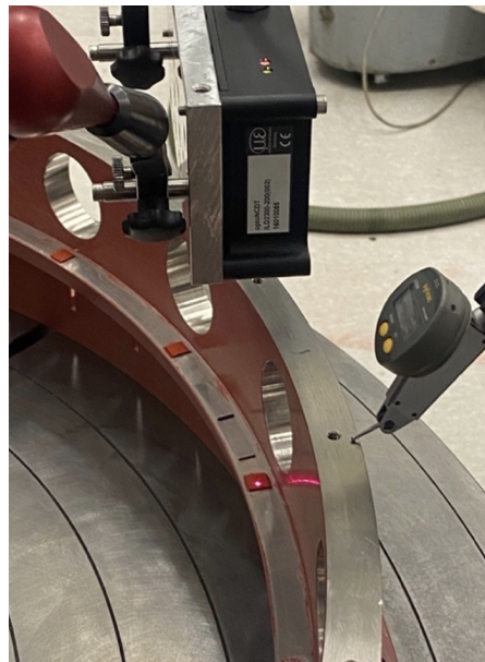
Figure 10: Image of the L1 axial pads being measured using the LDS, measurements were taken in the centre of the pad.
