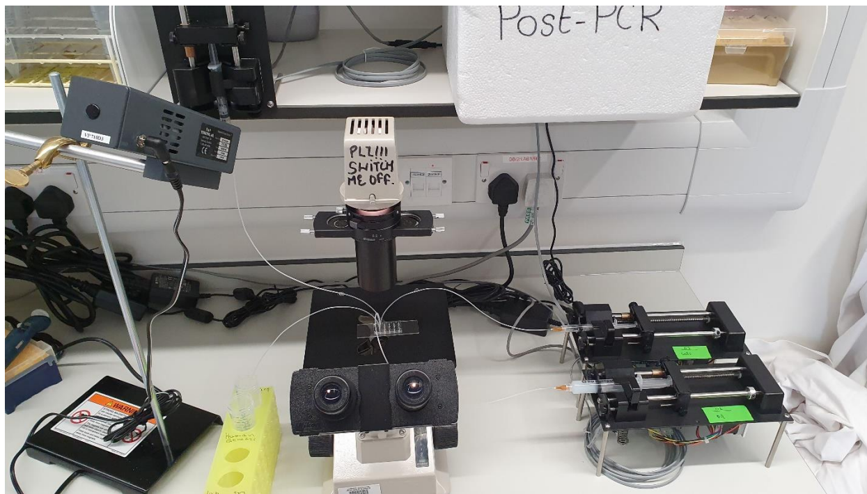
Figure 2.1: Photo of the working DroNc-seq setup. The three computer-controlled syringe pumps (top-left and right) were connected with tubing to the microfluidic device (centre) that was placed on a brightfield inverted microscope. A bead stirrer prevented the sedimentation of the barcoded beads. Flow rates were controlled by a computer (not shown), and the resulting emulsion was collected in a conical 15 mL tube. The device was constantly monitored for potential clogging.
