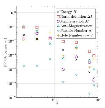
Figure 8. Dependence of different operators  $\langle O \rangle$  on the boundary MPS bond dimension  $\chi$  for the ground state in the odd parity sector. Shown are the relative errors compared to results at  $\chi = 100$ . Honeycomb Hubbard model with D = 12,  $L = 12 \times 6$ ,  $\kappa = 1$ , U = 2,  $\mu = 0.1$ , B = 0.01.
