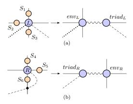
Figure 3. Splitting tensors into triads *triad* and the environments *env* for an update in x-direction. Symbology – small orange circles on indices: singular values; diamond: swap gate for fermionic PEPS.
