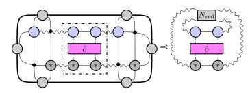
Figure 7. Calculating the expectation value of a two site operator  $\hat{o}$  in x-direction with a fermionic tensor network using boundary MPS. Wiggly lines denote a splitting of triads and environment tensors according to fig. 5 but without singular values S. Contraction of all tensors outside the dash dotted rectangle define the environment tensor  $N_{\rm red}$ .
