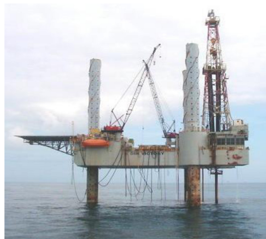
Fig. 1. Bethlehem JU 250 MS, jack-up offshore structure in the Gulf of Mexico ( www.offshoreenergytoday.com ).
