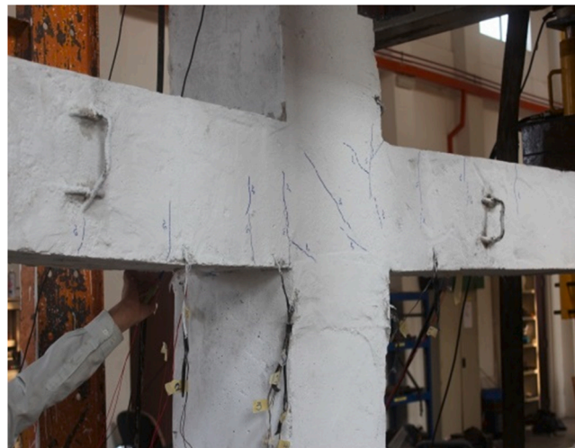
Fig. 14. Damage in the control connection in the experimental, J-0.
