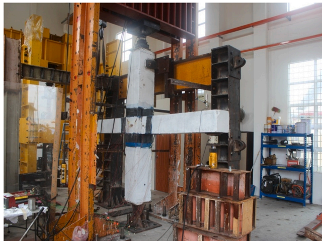
Fig. 9. Setup of experimental test for CFRP-strengthened connection, J-1.
