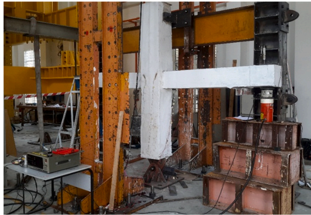
Fig. 8. Setup of experimental test for control connection, J-0.
