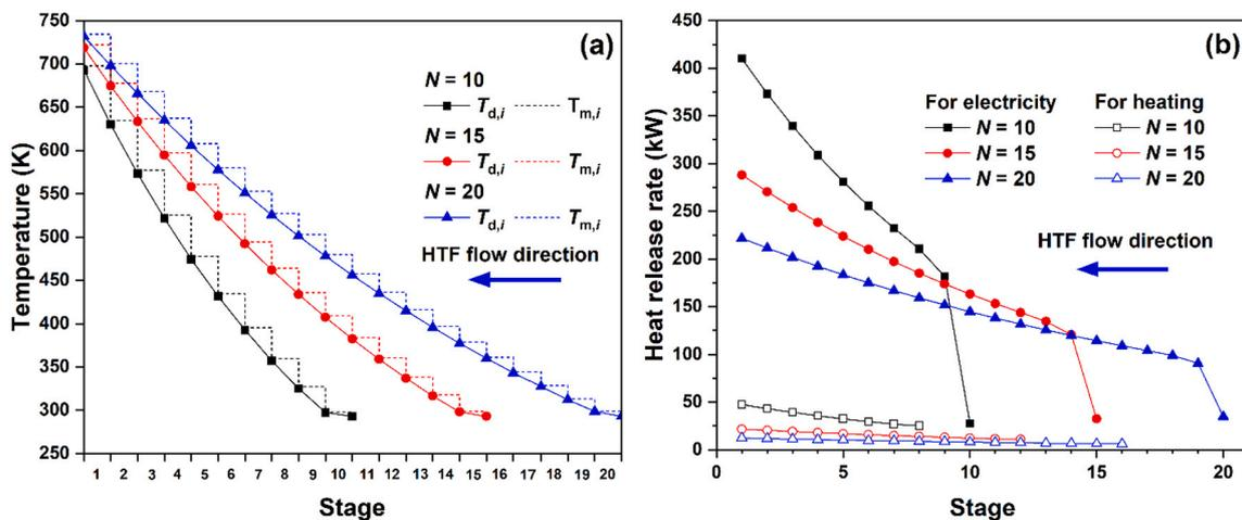
Fig. 11. Characteristics of each stage in CLHS during discharging: (a) melting and HTF outlet temperatures, and (b) heat release rate. Stage area  $A$  is 300 m<sup>2</sup>, HTF tube-side velocity  $v_{tube}$  is 5 m/s and total stage numbers  $N = 10, 15$  and 20 are considered.
