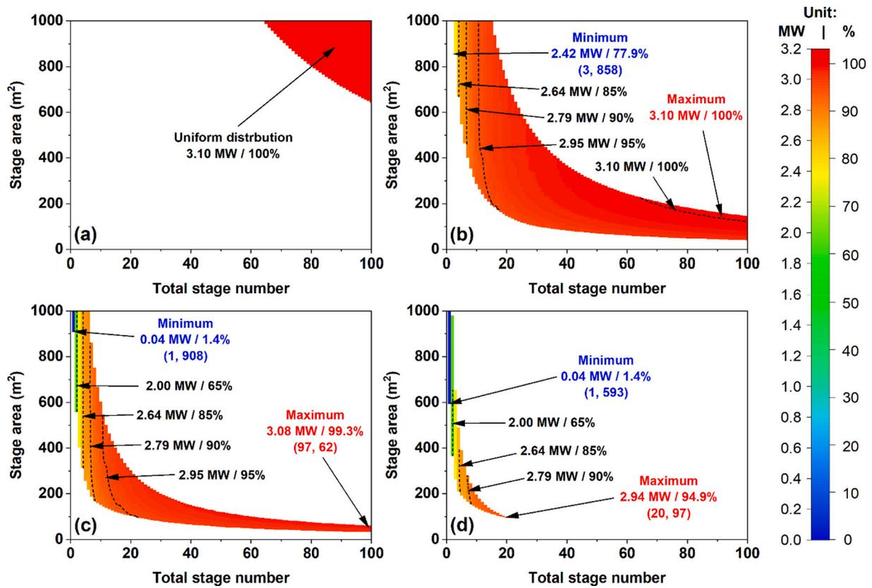
Fig. 8. Total heat release rate and RTE in CHP mode with respect to total stage number  $N$  and stage area  $A$ , with different HTF tube-side velocities  $v_{\text{tube}}$ : (a) 0.8 m/s, (b) 5 m/s, (c) 10 m/s, and (d) 15 m/s.
