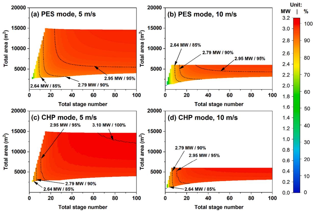
Fig. 10. Total heat release rate and RTE in different operational modes with respect to total stage number  $N$  and total area  $A_{tot}$ , with different HTF tube-side velocities  $v_{tube}$ : (a) PES mode and 5 m/s, (b) PES mode and 10 m/s, (c) CHP mode and 5 m/s, and (d) CHP mode and 10 m/s.
