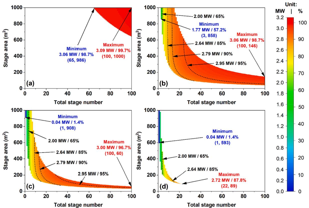
Fig. 7. Total heat release rate and RTE in PES mode with respect to total stage number  $N$  and stage area  $A$ , with different HTF tube-side velocities  $v_{\text{tube}}$ : (a) 0.8 m/s, (b) 5 m/s, (c) 10 m/s, and (d) 15 m/s.
