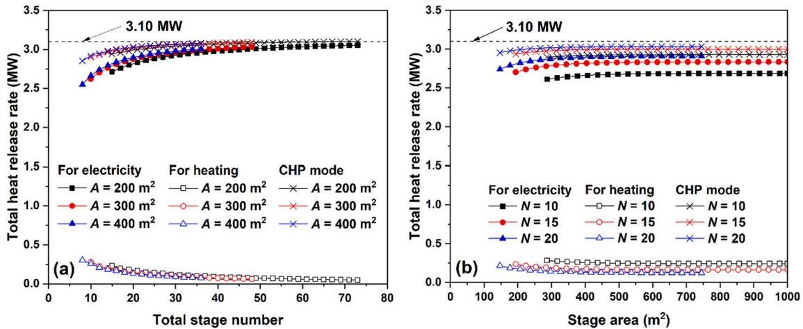
Fig. 9. Total heat release rate in CHP mode as a function of total stage number and stage area: (a) total stage number  $N$  varies from 1 to 80 and stage areas  $A$  of 200  $\text{m}^2$ , 300  $\text{m}^2$  and 400  $\text{m}^2$  are considered, and (b) stage area  $A$  changes from 10  $\text{m}^2$  to 1000  $\text{m}^2$  and total stage numbers  $N = 10, 15$  and 20 are investigated. HTF tube-side velocity  $v_{\text{tube}}$  is 5 m/s in all cases.
