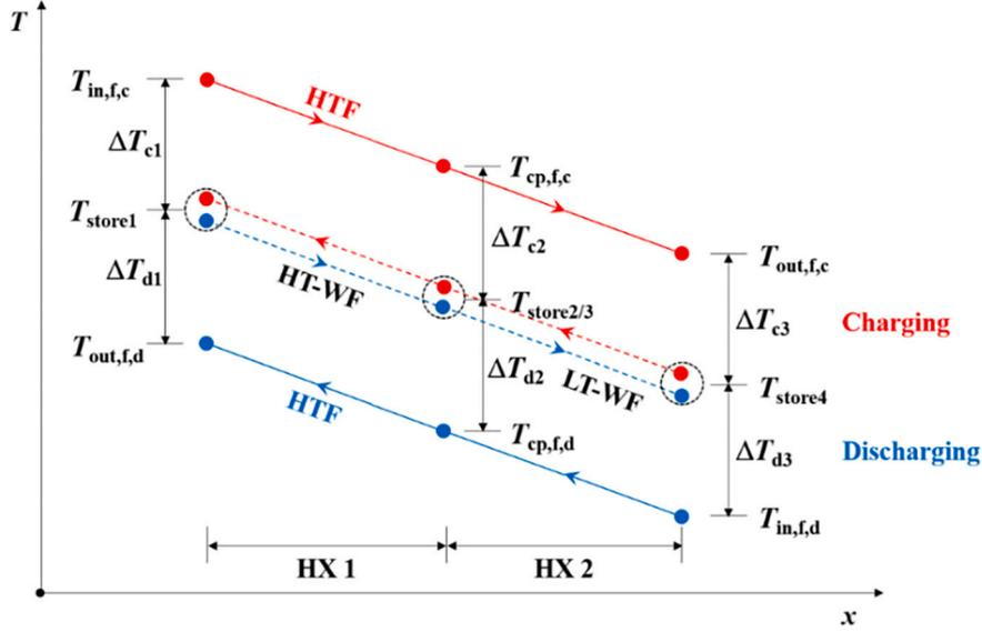
Fig. 3. Temperature distribution in liquid sensible-heat stores.
