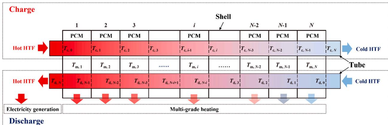
Fig. 1. Shell-and-tube type CLHS concept. (For interpretation of the references to colour in this figure, the reader is referred to the web version of this article.)
