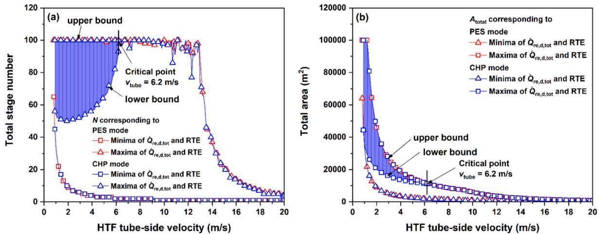
Fig. 14. Characteristics corresponding to the total heat release rate and RTE maxima and minima in PES and CHP modes as a function of HTF tube-side velocity  $v_{\text{tube}}$ : (a) total stage number  $N$ , and (b) total area  $A_{\text{tot}}$ .
