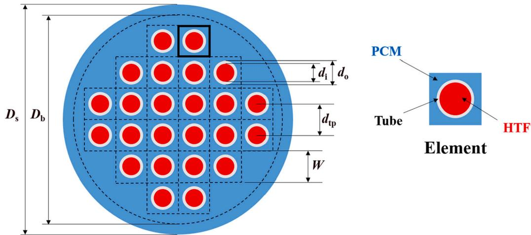
Fig. 2. Cross-section of shell-and-tube type CLHS.
