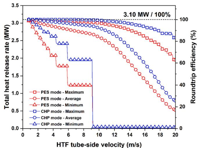
Fig. 13. Maximum, average and minimum of total heat release rate and RTE in PES and CHP modes as a function of HTF tube-side velocity  $v_{\text{tube}}$ . The maximum, average and minimum are calculated based on the results within the corresponding valid region of total stage number  $N$  and stage area  $A$ .
