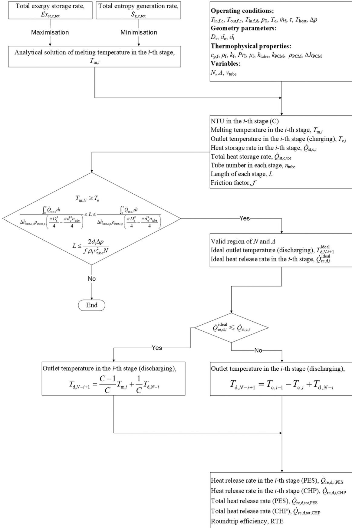
Fig. 3. Flowchart of model solution as implemented in MATLAB.
