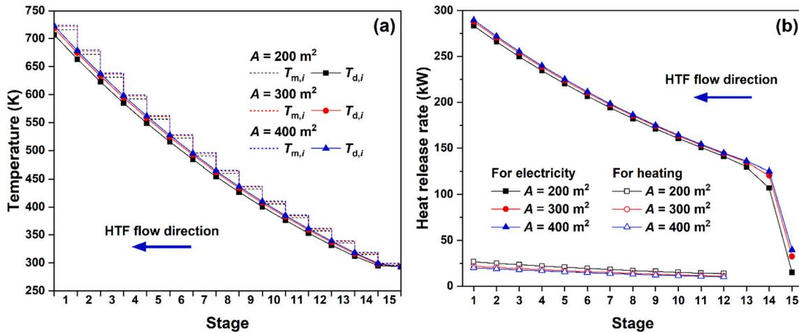
Fig. 12. Characteristics of each stage in CLHS during discharging: (a) melting and HTF outlet temperatures, and (b) heat release rate. Total stage number  $N$  is 15, HTF tube-side velocity  $v_{\text{tube}}$  is 5 m/s and stage areas  $A = 200 \text{ m}^2$ ,  $300 \text{ m}^2$  and  $400 \text{ m}^2$  are considered.
