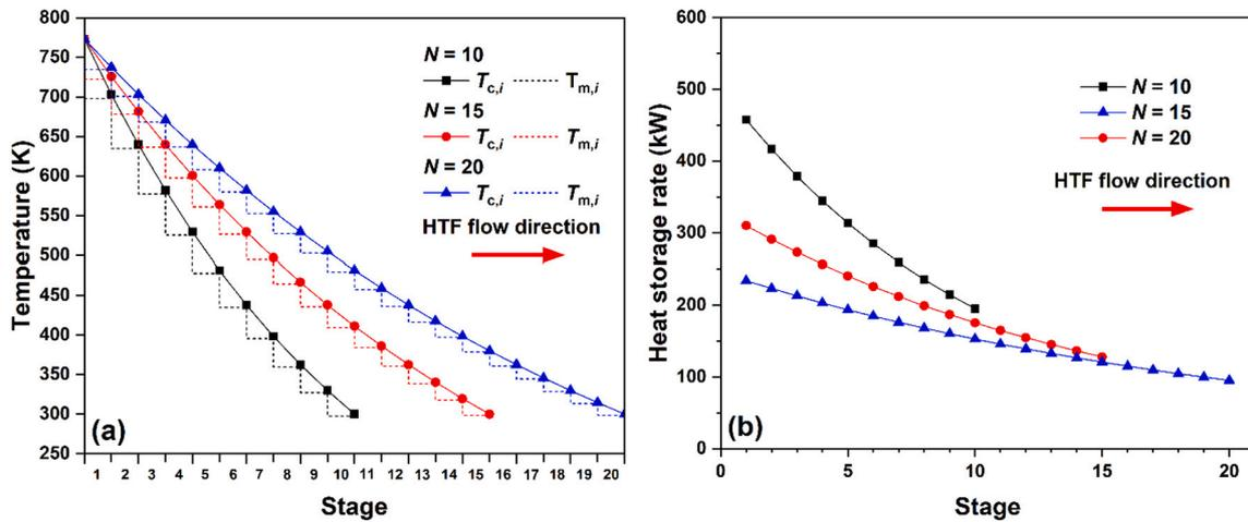
Fig. 5. Characteristics of each stage in CLHS during charging: (a) PCM melting and HTF outlet temperatures, and (b) heat storage rate. Stage area  $A$  is  $300 \text{ m}^2$ , HTF tube-side velocity  $v_{\text{tube}}$  is  $5 \text{ m/s}$  and total stage numbers  $N = 10, 15$  and  $20$  are considered.
