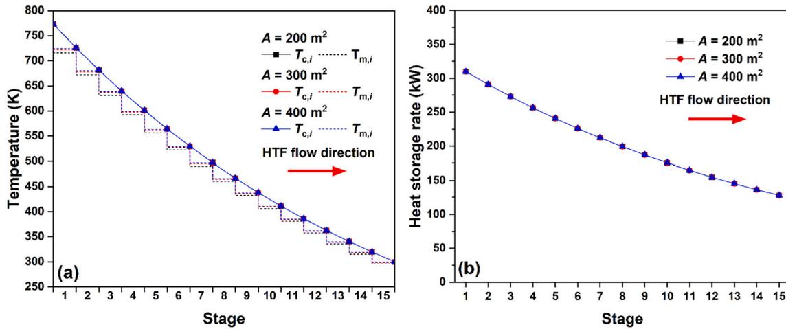
Fig. 6. Characteristics of each stage in CLHS during charging: (a) PCM melting and HTF outlet temperatures, and (b) heat storage rate. Total stage number  $N$  is  $15$ , HTF tube-side velocity  $v_{\text{tube}}$  is  $5 \text{ m/s}$  and stage areas  $A = 200 \text{ m}^2, 300 \text{ m}^2$  and  $400 \text{ m}^2$  are considered.
