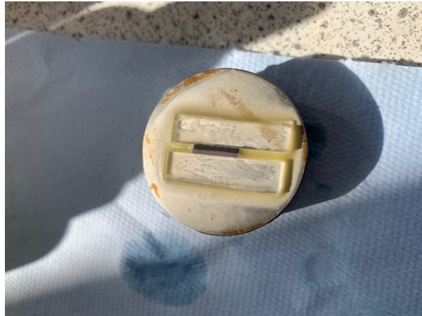
Figure 6.27 A photo of two exchanged sample stuck together fixed on the polishing block with wax during line scan sample preparation.
