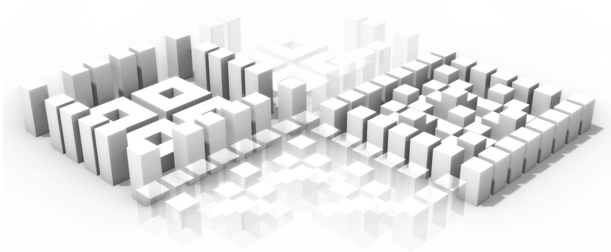
Figure 7.1: Recommendations for using courtyard block types. Conventional courtyard blocks are to be used in high-density areas (left), while residential solar blocks are to be used in compact areas (right).
