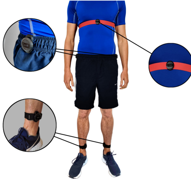
Figure 4-5: Subject wearing the Movesense IMU sensors on both ankles, hips and the chest.
