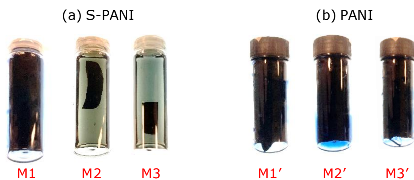
Fig. 3.8 Effect of DMF on membrane stability after two weeks.
