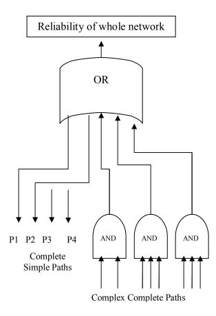
Figure 3 Dual fault tree representation of the whole network
