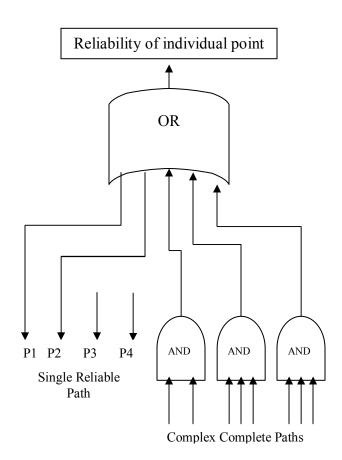
Figure 2 Dual fault tree representation of individual point
