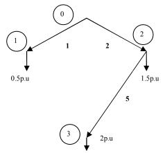
: The reliability of the whole network = R[path(1,3,5)] OR R[path (1) AND path(2,5)] OR R[path(2) AND path (1, 4)] =  $(R_1 R_3 R_5) OR (R_1 R_2 R_5) OR (R_2 R_1 R_4)$
