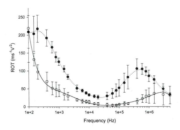
Figure 4.2. Electrorotation spectra of carboxylated elliptical latex particles suspended in  $430\,\mu\text{Sm}^{-1}$  PBS solution after preparation ( ) and after 24 hours storage at 4°C ( ) (for a sample of 13 particles). Error bars represent the 95% confidence of the standard deviation.
