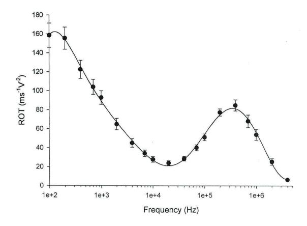
Figure 6.7. Electrorotation spectra of latex particles coated with primary antibodies, secondary antibodies and tertiary gold-conjugated antibodies. Error bars are the 95% confidence of the standard deviation.
