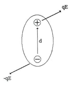
Figure 2.12. Force components creating a net torque on a dipole, m = qd, in an electric field. The positive and negative charges generate forces in opposite directions, these generate a torque as the dipole tries to align itself with the electric field.
