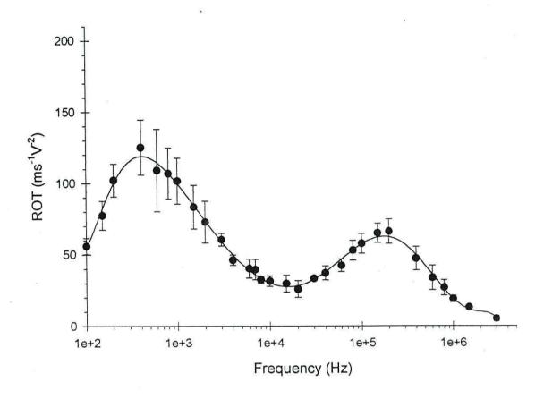
Figure 5.6. Electrorotation spectrum of latex beads coated with 20µl of E. coli antibody in 500  $\mu Sm^{-1}$  PBS solution, sample of 6 particles.
