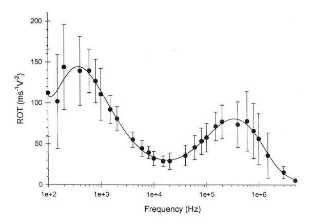
Figure 5.7. Electrorotation spectrum of latex beads coated with 25 $\mu$ l of *E. coli* antibody in 500  $\mu$ Sm<sup>-1</sup> PBS solution, sample of 9 particles.
