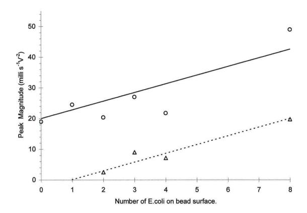
Figure 5.17. Change in magnitude of the high frequency peak  $\bigcirc$  ) and anti-field peak  $(\triangle)$  for the addition of non-viable E. coli to the surface of separate antibody-coated beads.
