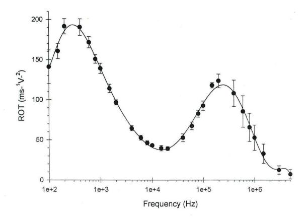
Figure 5.5. Electrorotation spectrum of latex beads coated with 15µl of *E. coli* antibody in 500  $\mu Sm^{-1}$  PBS solution, sample of 11 particles.
