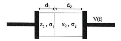
Figure 2.7. Parallel plate capacitor with an applied voltage of frequency, f. The plates are of surface area A. The gap is filled by two dielectrics of thickness  $d_1$  and  $d_2$ , with permittivities  $\varepsilon_1$  and  $\varepsilon_2$  and conductivity's  $\sigma_1$  and  $\sigma_2$ .
