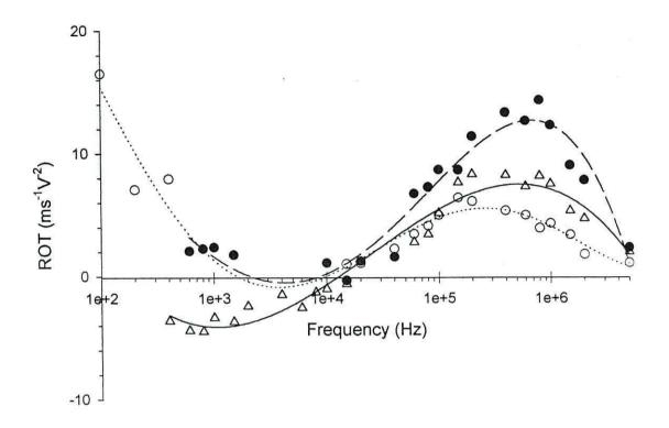
Figure 5.20. Electrorotation spectra obtained on addition of one (---), two (--) and three (---) viable *Bascillus subtilis* to the surface of separate antibody-coated beads.
