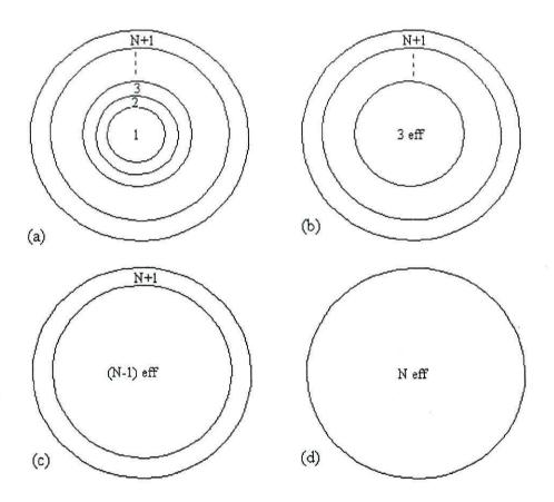
Figure 2.15. A smeared out spherical shell approach to determine the effective permittivity of a sphere consisting on N shells. (a) to (d) represent the effect of smearing the shells.
