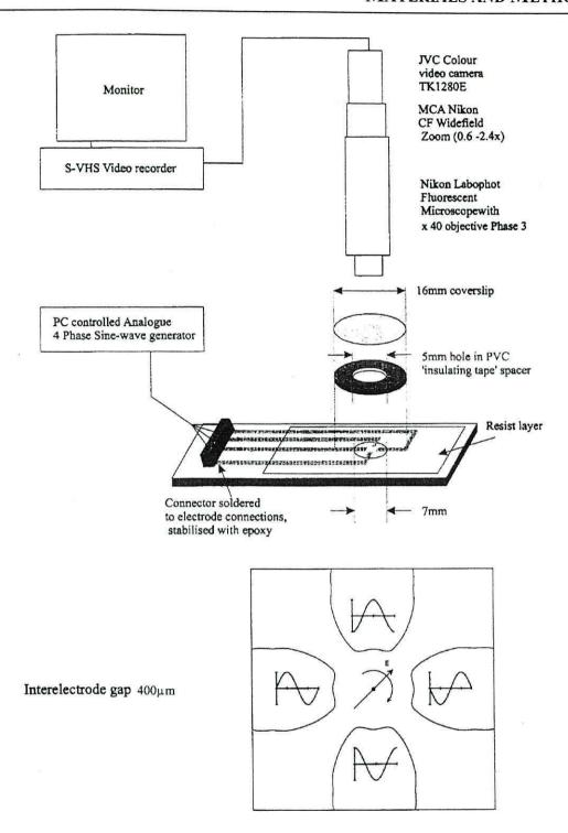
Figure 3.18. Electrorotation experiment setup, with a view of the 'bone' electrodes.
