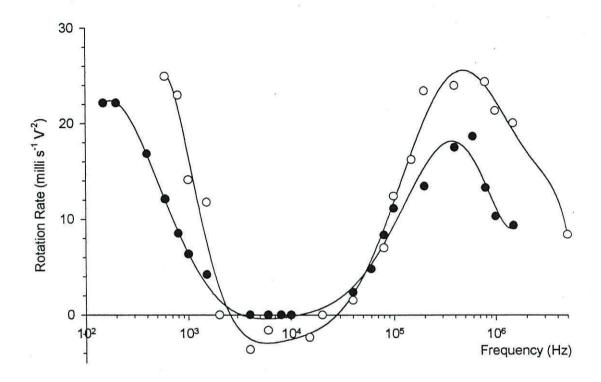
Figure 5. Electrorotation spectra obtained on addition of one non-viable ( $\odot$ ) and two non-viable ( $\bigcirc$ ) E. coli to the surface of separate antibody-coated beads.
