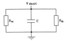
Figure 2.1 Equivalent circuit of a real capacitor.
