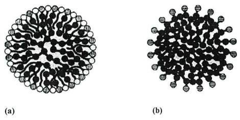
Figure 3.4. Illustration of the latex particle, (a) before ion exchange, with sodium and potassium counter ions in the solution, (b) after ion exchange, with water-soluble electrolyte removed.
