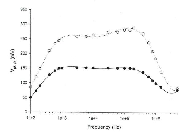
Figure 4.4. Graph indicating the change in medium conductance (voltage) of samples of elliptical latex beads with carboxylate surface functional groups in ultra-pure water after preparation ( $\bullet$ ) and after 23 hours storage at  $4^{\circ}C(\bigcirc)$ .
