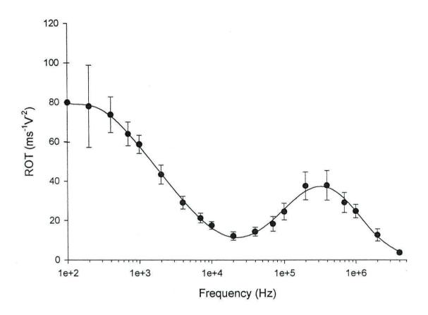
Figure 6.4. Electrorotation spectra of latex particles coated with primary antibodies and secondary antibodies. Error bars are the 95% confidence of the standard deviation.
