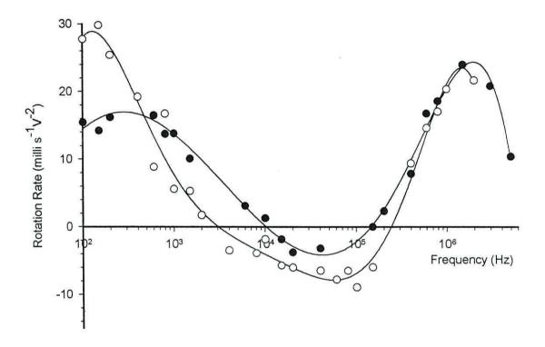
Figure 5.12. Electrorotation spectra obtained on addition of one viable ( $\bigcirc$ ) and two viable ( $\bigcirc$ ) E. coli to the surface of separate antibody-coated beads.
