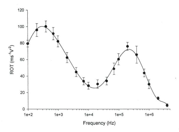
Figure 6.3. Electrorotation spectra of latex particles coated with primary antibody. Error bars are the 95% confidence of the standard deviation.
