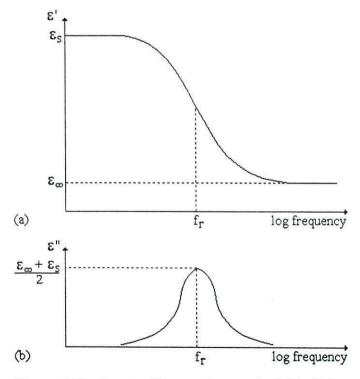
Figure 2.3 Graphs illustrating typical (a) dielectric permittivity and (b) loss with frequency.
