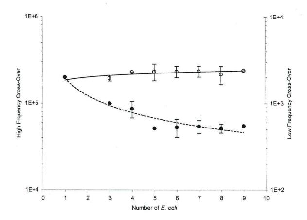
Figure 5.13. Change of the high frequency cross-over ( $\bigcirc$ ) and low frequency cross-over ( $\bigcirc$ ) for the addition of up to nine viable *E. coli* to the surface of separate antibody-coated beads. Error bars indicate the maximum and minimum deviations.
