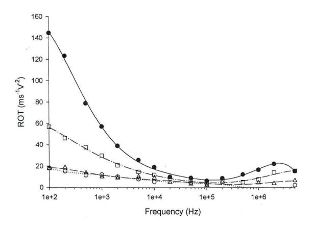
Figure 4.5. Electrorotation spectra of elliptical latex particles with carboxylate surface functional groups suspended in a range of relatively high conductivity normal PBS solution. The conductivities were:  $10 \text{ mSm}^{-1}$  ( $\bigcirc$ ),  $25 \text{ mSm}^{-1}$  ( $\square$ ),  $50 \text{ mSm}^{-1}$  ( $\triangle$ ) and  $75 \text{ mSm}^{-1}$  ( $\bigcirc$ ).
