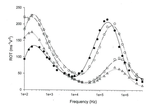
Figure 4.6. Electrorotation spectra of elliptical latex particles with carboxylate surface functional groups suspended in a range of relatively low conductivity normal PBS solution. The conductivities were: ultra-pure water (at 150  $\mu Sm^{-1})$   $\bigcirc$ ), 430  $\mu Sm^{-1}$  (  $\square$ ), 620  $\mu Sm^{-1}$  (  $\bigcirc$ ) and 2100  $\mu Sm^{-1}$  (  $\triangle$ ).
