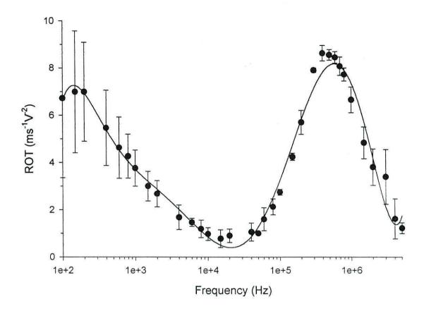
Figure 6.2. Electrorotation spectra of primer two. The error bars represent the minimum and maximum deviations only.
