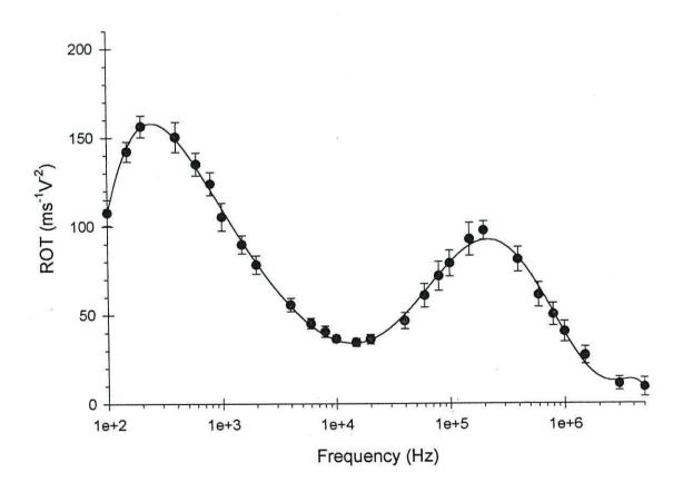
Figure 5.4. Electrorotation spectrum of latex beads coated with  $10\mu l$  of *E. coli* antibody in  $500 \, \mu Sm^{-1}$  PBS solution, sample of 13 particles.
