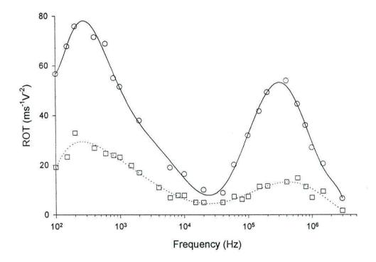
Figure 5.9. Electrorotation response of *E. coli* antibody coated latex beads, freshly prepared ( $\bigcirc$ ) and after one month of refrigerated storage ( $\square$ ), suspended in 500  $\mu$ Sm<sup>-1</sup> PBS solution.
