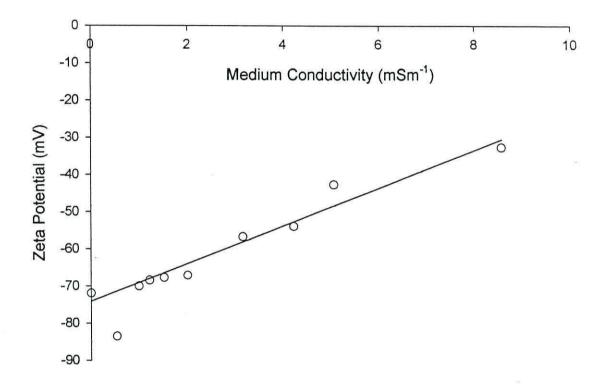
Figure 4.8. Variation in the Zeta potential, of carboxylated elliptical latex particles, with increasing suspending medium conductivity.
