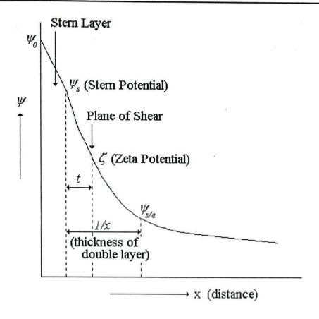
Figure 2.14. Potential distribution for the Gouy-Chapman-Stern model of the electrical double layer as a function of the distance from the solid-liquid interface.
