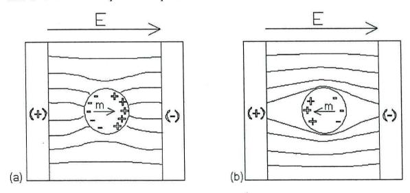
Figure 2.8. The distribution of electric charges induced at the surface of a particle and the direction of the resulting dipole moment, m. (a) Where the polarisability of the particle is greater than the surrounding medium, and (b) where the polarisability of the particle is less than the surrounding medium.
