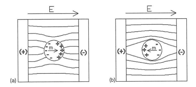
Figure 2.9. Two particles in a non-uniform field. The particle on the left is more polarisable than its suspending medium and is attracted to the high field region, at the pin electrode. The particle of low polarisability, on the left, is repelled from the high field area.
