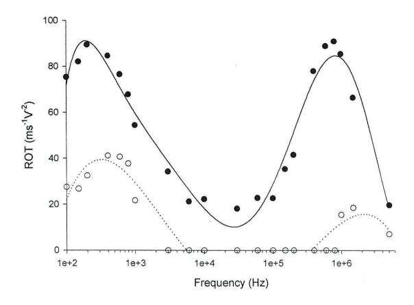
Figure 4.3. Electrorotation spectra of carboxylated elliptical latex particles suspended in ultra-pure water. Freshly prepared ( $\bigcirc$ ) and after 23 hours storage at  $4^{\circ}C(\bigcirc)$ .
