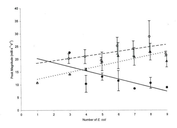
Figure 5.14. Change in magnitude of the high frequency peak  $(-\Theta^-)$ , low frequency peak  $(-\Phi^-)$ , and anti-field peak  $(-\Phi^-)$  for the addition of up to nine viable  $E.\ coli$  to the surface of separate antibody-coated beads. Error bars indicate the maximum and minimum deviations.
