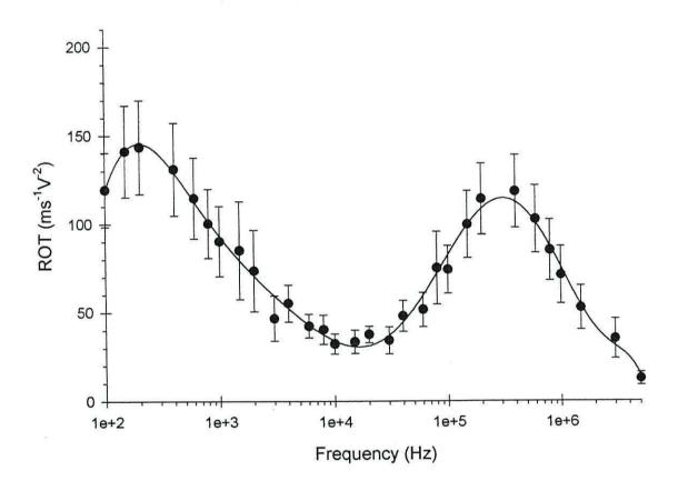
Figure 5.3. Electrorotation spectrum of latex beads coated with  $5\mu l$  of *E. coli* antibody in  $500 \, \mu Sm^{-1}$  PBS solution, sample of 12 particles.
