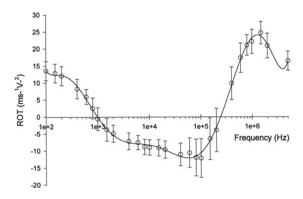
Figure 5.18. Electrorotation spectra of antibody coated beads with four viable *E. coli* attached to the surface. The error bars are the 95% confidence of the standard deviation, based on a sample of 21 beads.
