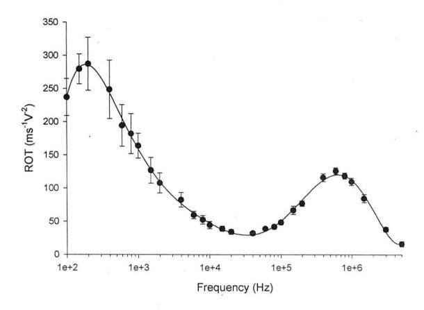
Figure 4.1. Electrorotation spectra of elliptical latex particles with carboxylate surface groups suspended in  $430 \,\mu\text{Sm}^{-1}$  PBS solution (where n = 7 beads). Error bars represent the 95% confidence of the standard deviation.
