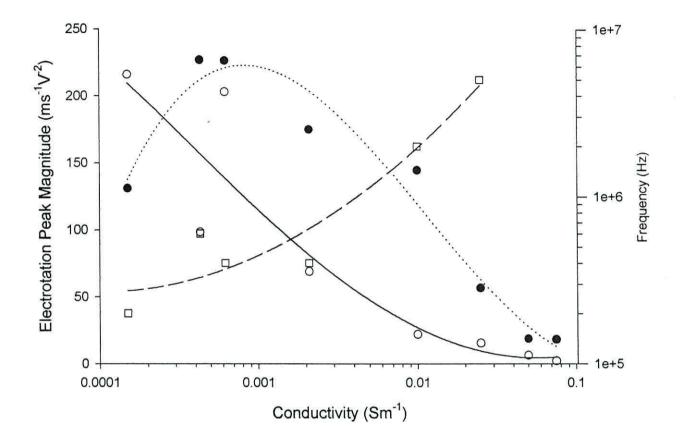
Figure 4.7. Summary of the changes in the high frequency peak magnitude ( $\bigcirc$ ) and frequency ( $\square$ ) and the low frequency peak magnitude ( $\bigcirc$ ) for carboxylated elliptical particles suspended in increasingly conductive PBS solutions.
