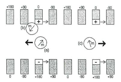
Figure 2.13. (a) Motion expected for a particle that is more polarisable than its suspending medium. (b) A cell trapped by positive dielectrophoresis. (c) Motion expected for a particle that is less polarisable than its suspending medium.
