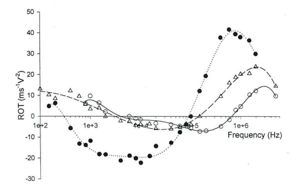
Figure 5.11. Change with time of electrorotation spectra of antibody coated beads with three E. coli bound to the surface.  $(\bigcirc)$  are the results after 20 minutes,  $(\bigcirc)$  after one hour and  $(\bigcirc)$  after two hours from the start of the experiment.
