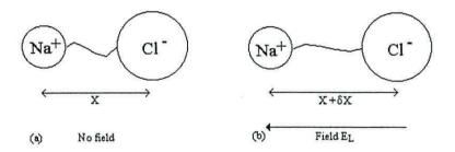
Figure 2.5 Action of an electric field on an ionic molecule.
