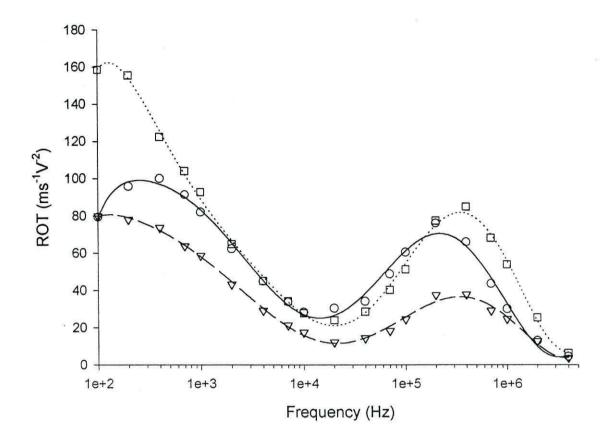
Figure 6.8. Electrorotation spectra of latex particles coated with only primary antibody  $(\bigcirc)$ , with additional secondary antibody  $(\bigtriangledown)$  and with a tertiary gold-conjugated antibody added  $(\Box)$ .
