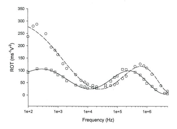
Figure 4.9. Electrorotation spectra of elliptical latex particles with additional carboxylate surface functional groups ( $\bigcirc$ ) and no additional surface functional groups ( $\square$ ) suspended in 430  $\mu Sm^{-1}$  PBS solution.
