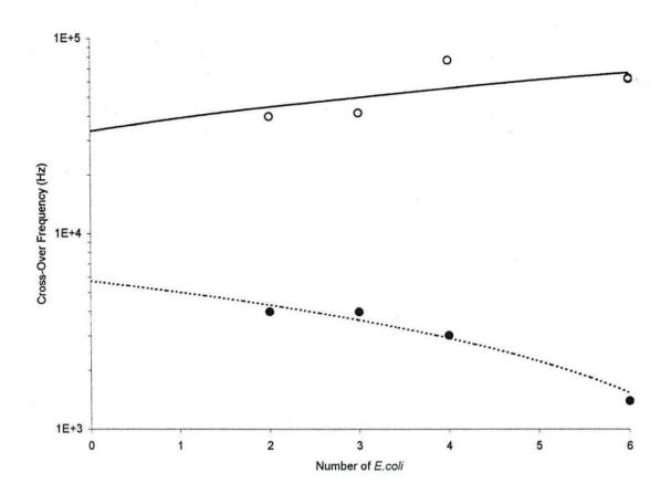
Figure 5.16. Change of the high frequency cross-over ( $\bigcirc$ ) and low frequency cross-over ( $\bigcirc$ ) for the addition of up to six non-viable *E. coli* to the surface of separate antibody-coated beads.
