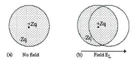
Figure 2.4 Diagram to describe the action of an electric field on an atom, electronic polarization.
