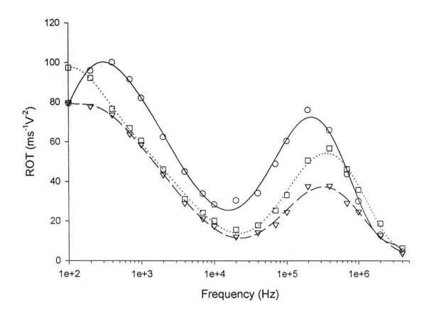
Figure 6.6. Electrorotation spectra of latex particles coated with only primary antibody  $(\bigcirc)$ , with additional secondary antibody  $(\bigtriangledown)$  and with a tertiary FITC-conjugated antibody added  $(\Box)$ .
