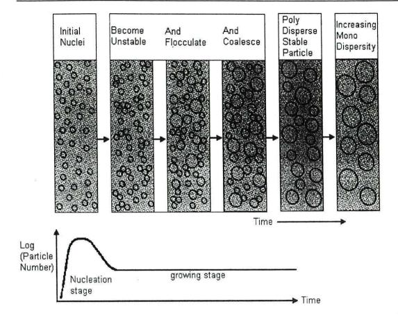
Figure 3.2. Nucleation and growth of the particles.
