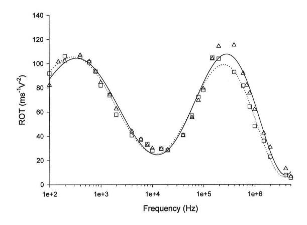
Figure 4.10. Electrorotation spectra of elliptical latex particles ( $\square$ ) and peanut shaped latex particles ( $\triangle$ ) with no additional surface functional groups suspended in 430  $\mu Sm^{-1}$  PBS solution.
