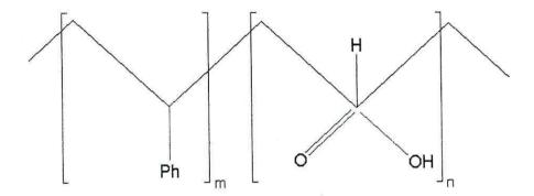
Figure 4.11. Chemical arrangement of the polystyrene latex beads. Ph represent the phenyl groups and m and n are the number of repeating units.
