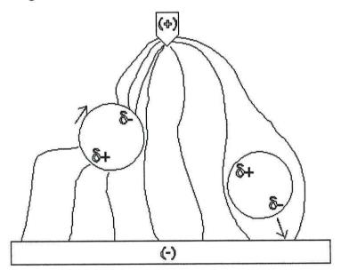
Figure 2.10. The net force on a dipole given by m = qd in a non-uniform field. The electric field vectors show the direction and magnitude of the electric field at the positive and negative charges.
