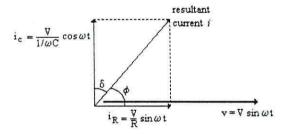
Figure 2.2 Phasor diagram for the equivalent circuit of a 'real' capacitor.
