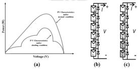
**Figure 6** PV Characteristics under shading and normal conditions (a), normal and shaded condition of the PV cell (b) & (c)
