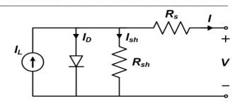
Figure 2 Fundamental equivalent circuit model of PV unit
