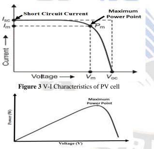
Figure 4 P-V characteristics under constant irradiation and temperature
