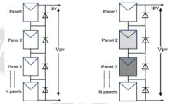
Figure 5 Connection of bypass diodes for each PV cell
