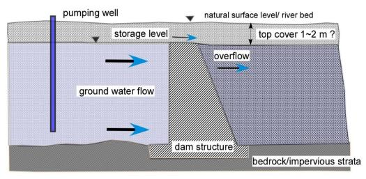
Figure 1. Typical scanrio for a subsurface dam
