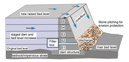
Figure 2. Scamatic repsresentation of a staged sand storage dam
