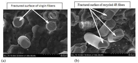
**Figure 5:** Fractured fibres in injection molded virgin material and 4R material after tensile test are shown in figures (a) and (b), respectively.
