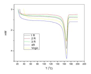
Figure 2: DSC of GFRPP samples showing no variations in Tg with recycling.
