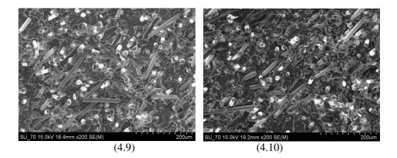
**Figure 4:** 4.1-4.10 SEM micrographs of various GFRPP fractured specimens. 4.1 and 4.2 for virgin material, 4.3 and 4.4 for 1 R, 4.5 and 4.6 for 2R, 4.7 and 4.8 for 3R, 4.9 and 4.10 for 4R.
