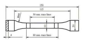
Figure 1:Standard tensile testing specimen [12].
