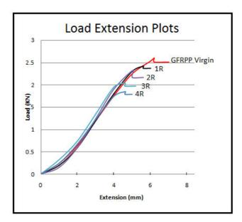
Figure 3: The average load – extension curves of virgin and four recycled generations.
