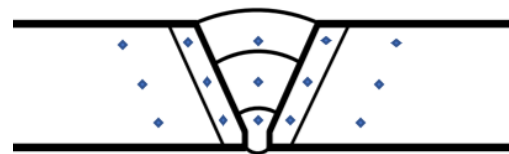
Gambar 4. Coupon hardness vickers test
