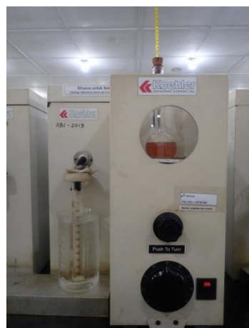
Gambar 2. Proses Distilasi bahan bakar cair
