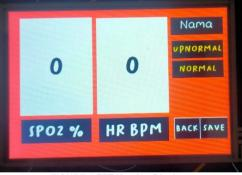
FIGURE 6 TFT Nextion Display
