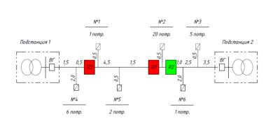
Figure 1– a) - Scheme of the ring feeder before the installation of reclosers: №1, №4, №5 – numbers of consumers of line 1 from substation 1; No. 2, No. 3, No. 6 - numbers of taps of line 2 from substation 2; b) - ring feeder diagram after installation of reclosers: R1, R2, R3 - reclosers.
