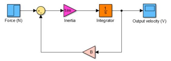
Figure 2 The car Simulink model.
