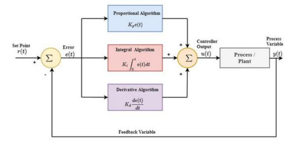
Figure 4 PID controller block diagram.
