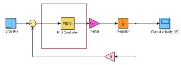
Figure 5 PID controller block diagram.
