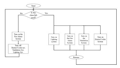
Figure 12: Flow diagram for the working of the second subsystem
