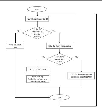
Figure 11: Flow diagram for the working of the first subsystem
