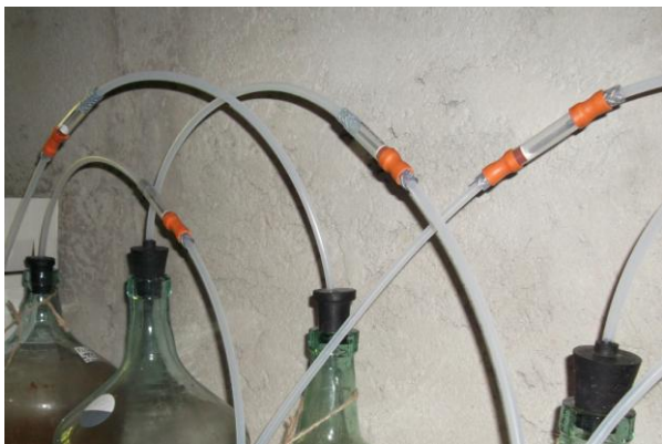
Figure 1 Capturing of exhaust CO 2 and compounds in Tamaioasa romaneasca fermentation process
