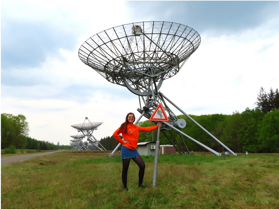
Figure 1.7: Six of the Westerbork Synthesis Radio Telescope dishes with an FRB hunter for scale. The white boxes at the focal point of each dish are the Apertif PAFs.
