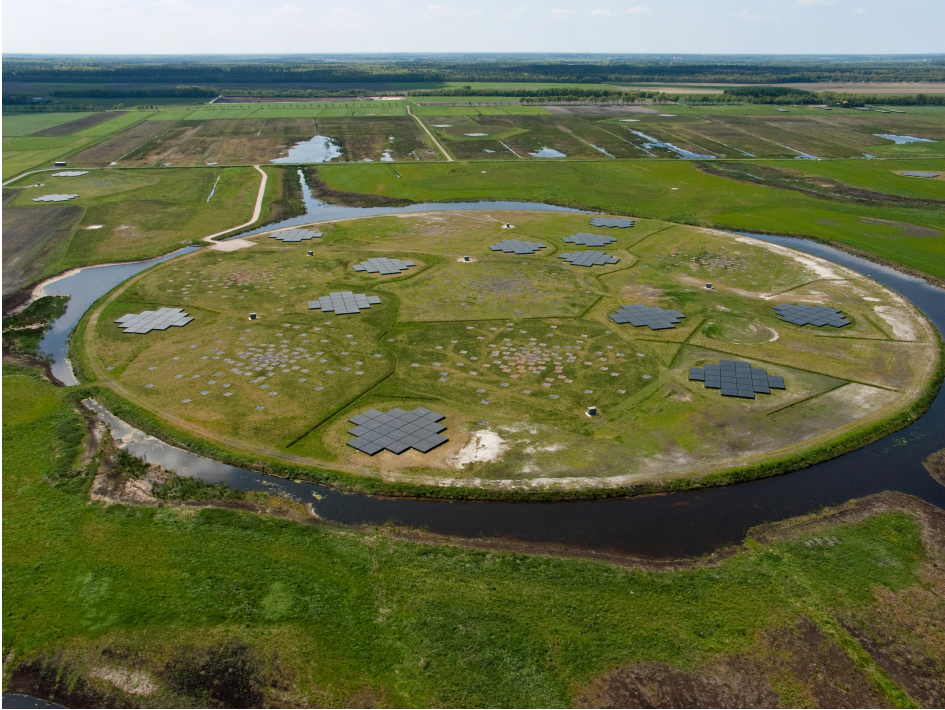
Figure 1.8: Drone image of the LOFAR core, known as “Superterp”. The HBA are the compact black tiles, and the LBA the scattered dipoles. Image credit: LOFAR / ASTRON.
