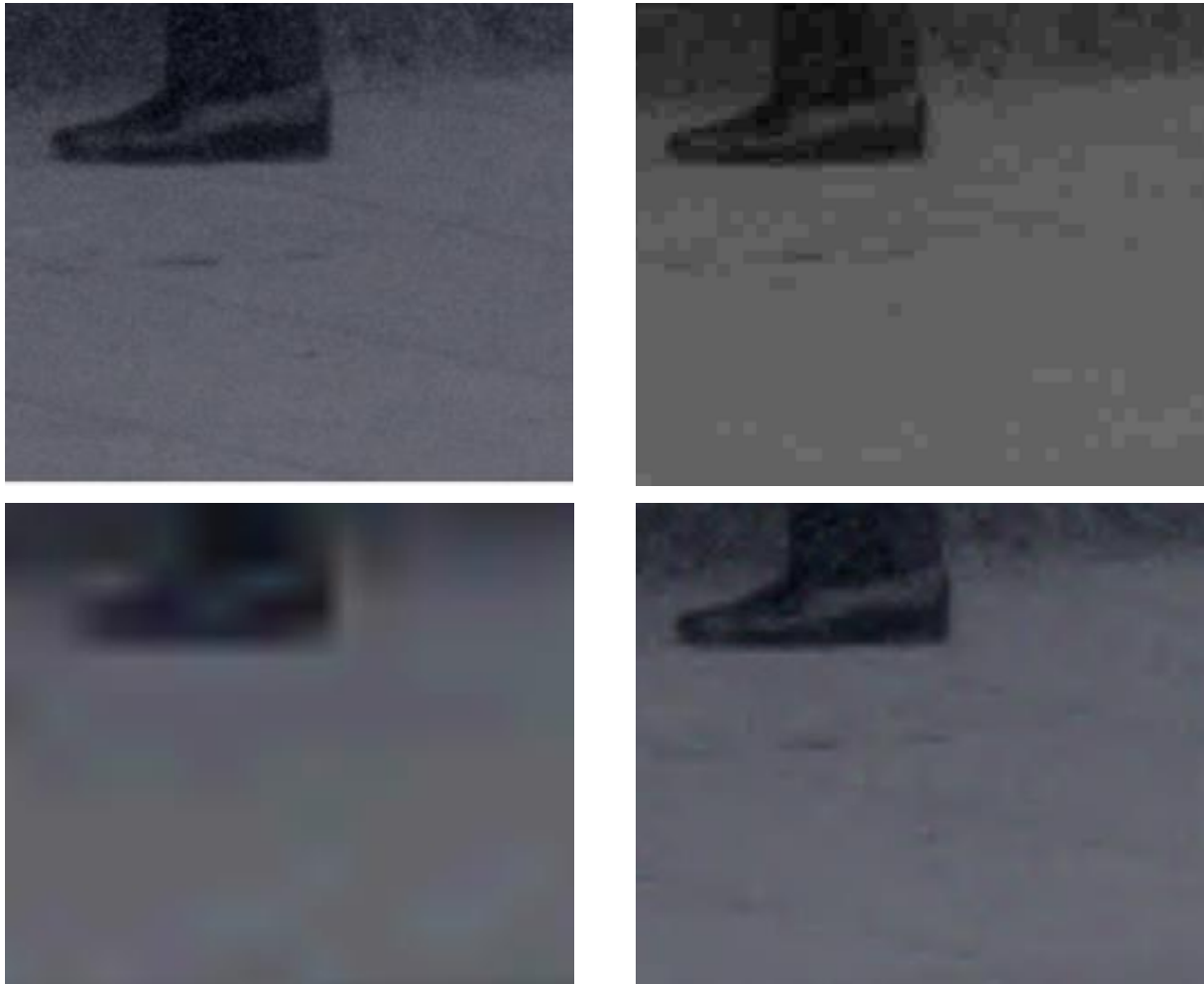
Figure 35 Clockwise from top left: Close-up shots of the Charles mort ou vif frame. A) Original image as lossless TIFF. B) Image compressed as JPEG with DCT compression. C) Image compressed as JPEG 2000 with wavelet compression, higher quality. D) Image compressed as JPEG 2000 with wavelet compression, lower quality, where the too high compression rate has extensively blurred it.
