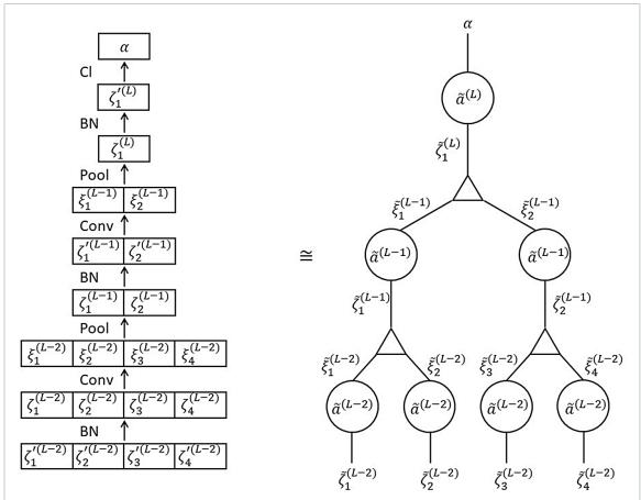
Figure 1. The neural network architecture used in this paper (left), and its tensorial description (right). The triangles represent the delta tensor implementing the same-channel product pooling (8). The circles represent the matrix multiplication as in (6).
