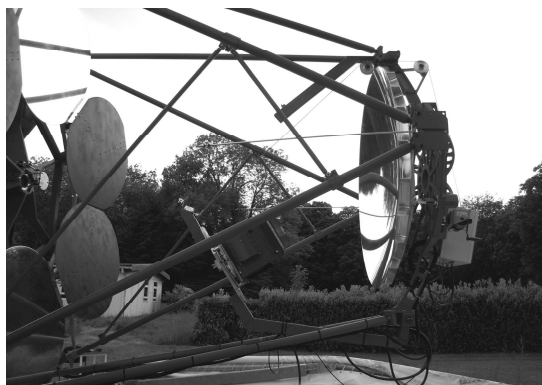
Figure 5: The GCT camera removal mechanism. The camera is in an intermediate position between a lower position (at less than 1 meter from the ground) and its observing position in front of the secondary mirror at the right. A pulley behind the secondary mirror allows the camera to go up or down. © 'The GCT Consortium'.
