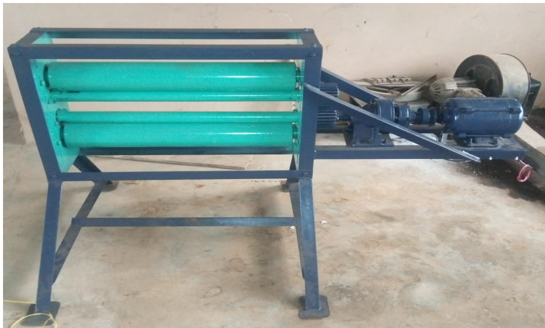
Fig. 4 Pictorial view of the Fabricated one-stand hot tandem rolling mill.
