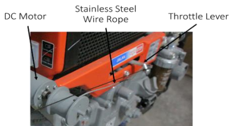
Figure 18. G3000 throttle lever mechanical modification
