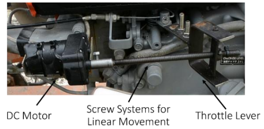
Figure 17. G1000 throttle lever mechanical modification
