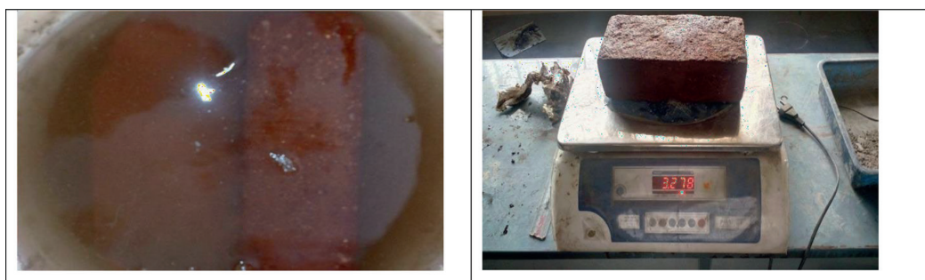
Figure 9. Sawdust bricks during water absorption test.
