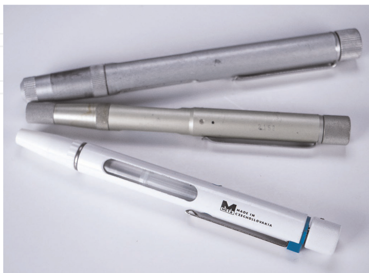
Figure 14. First insulin pens MADI (MAnual Device for Insulin) developed at Palacký University Olomouc in 1983–1990 [20, 21, 78] MADI 5/5 ml (above), MADI 7/2 ml—used in this study (middle), MADI 8/3 ml (below). Photo V. Kupčík, www.diabetesmuseum.cz .
