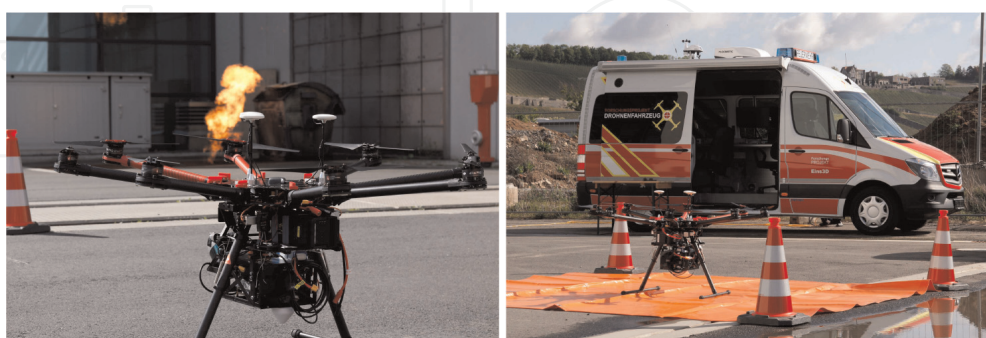
Figure 2. UAV with mounted mapping payload in front of simulated facade fire (left) and the firefighter command vehicle (right).
