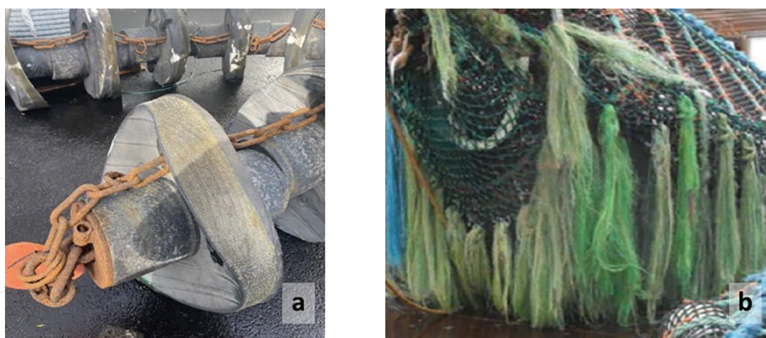
Figure 1. Worn-out rockhopper gear (a) and dolly rope used to protect the trawl (b). Photo: SINTEF.
