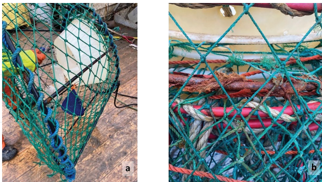
Figure 3. Snow crab pot (a), with cracked coating (b). Photo: SINTEF.
