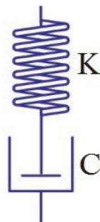
Figure 4. Maxwell mechanical model (spring and dashpot in series).
