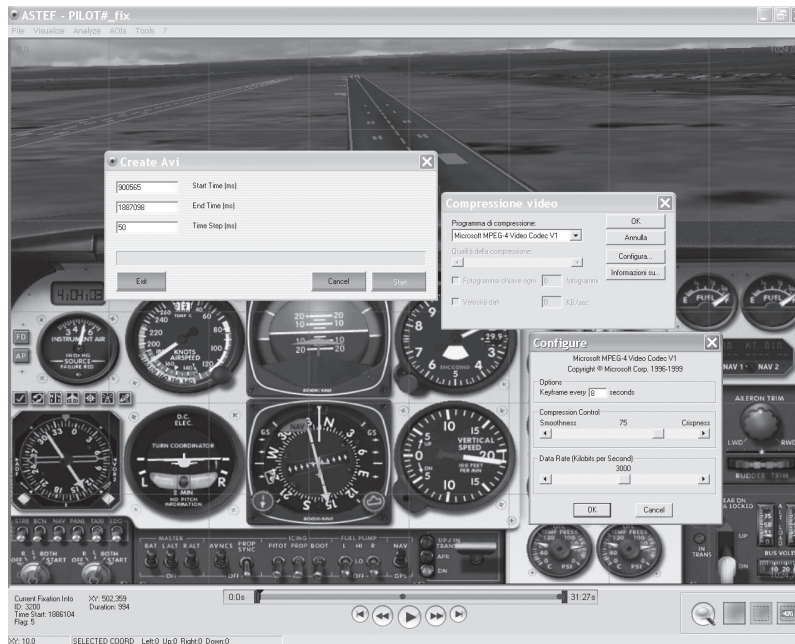
Figure 2. Example of scanpath clip exporting. Create AVI: Setup of start time and end time of recording. Compressione video: the choice of the codec for video compression. Configure: the configuration of the codec parameters.
