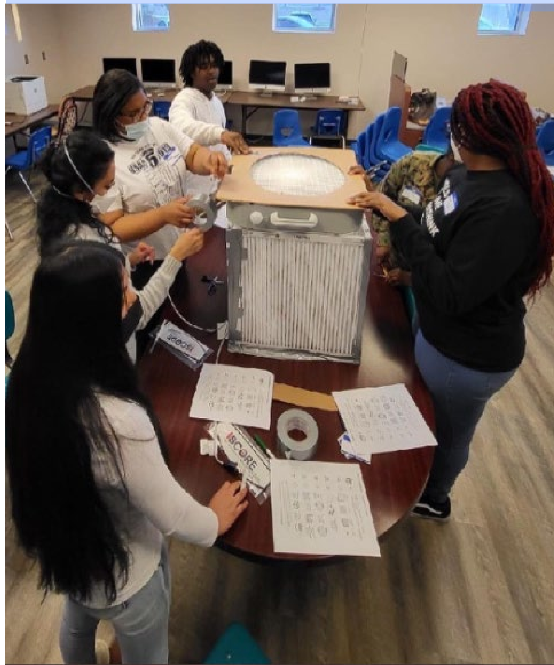
SCORE students building a #corsirosenthalbox as part of a COVID-19 lesson on layered mitigation
