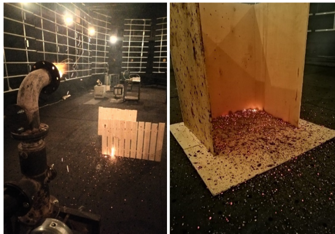
Figure 7. Images of ignition observed for fence and wood decking.
