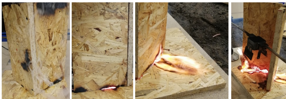
Figure 3. Set of images on ignition of a structure made of wood with particles.
