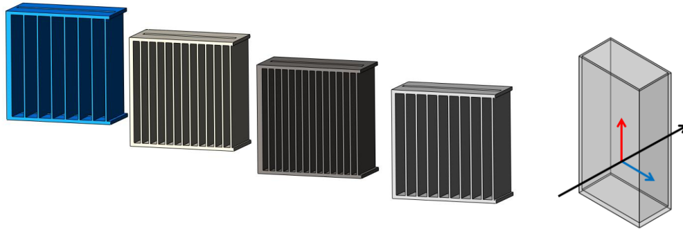
Figure 1. Scheme of a 3D printed insets and an overview of a cuvette with a polarization of THz radiation.
