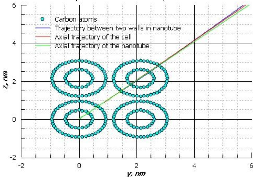
**Figure 4.** Trajectories of motion of water molecules in a system of 4 double-walled nanotubes at a speed of 450 m / s in the YZ plane.
