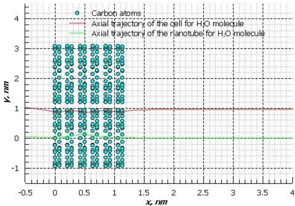
**Figure 3.** Trajectories of motion of water molecules in a system of 4 double-walled nanotubes at a speed of 450 m / s in the XY plane.
