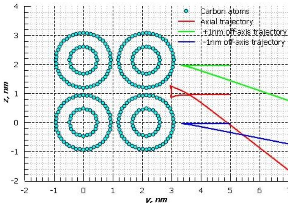
Figure 5. Three trajectories of motion of water molecules: axial, +1nm off-axis and -1nm off-axis variant
