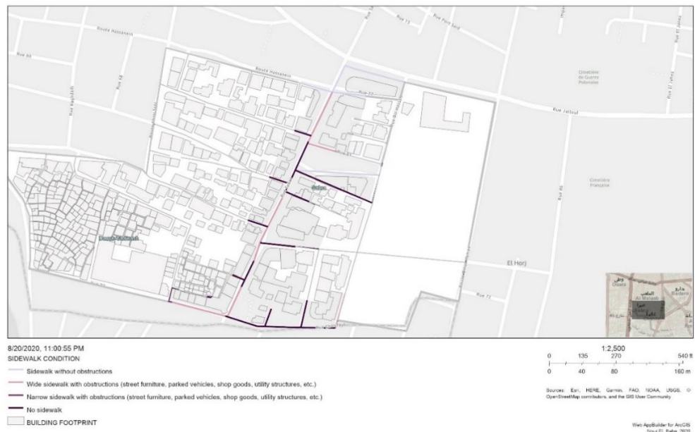
Fig.18: Showing the Sidewalk conditions along Sabra Commercial Urban Corridor Source: Map exported from Geoportal and analyzed by the Author, Data by (UN-Habitat–UNICEF, 2018)
