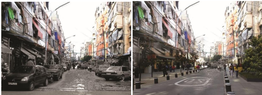
Fig.20: Showing before and after photo of Sabra Commercial Urban Corridor showing the proposed guideline in creating buffers between pedestrian and vehicular traffic
