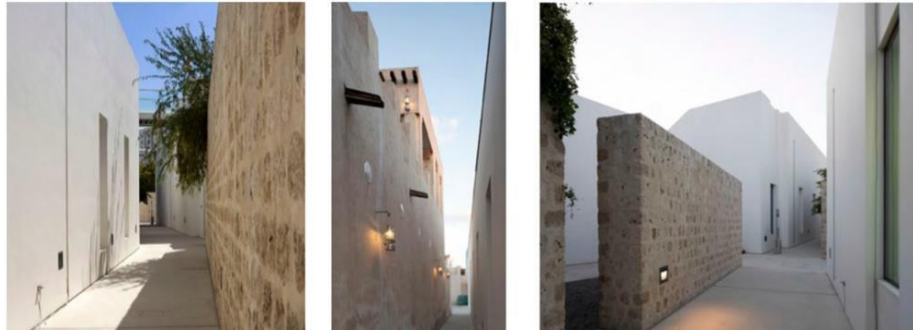
Fig.7: SAF narrow streets and irregular spaces allowing wind circulation. (Ibrahim. I & El Tarabishi. F, 2021)
